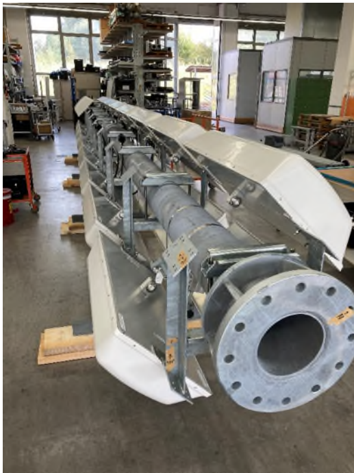
picture 3, left: Pre-assembly of the UHF antenna system at the KATHREIN plant in Rohrdorf, Germany
